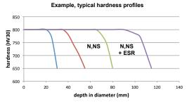
For high hardness depth, the N grade is required.
