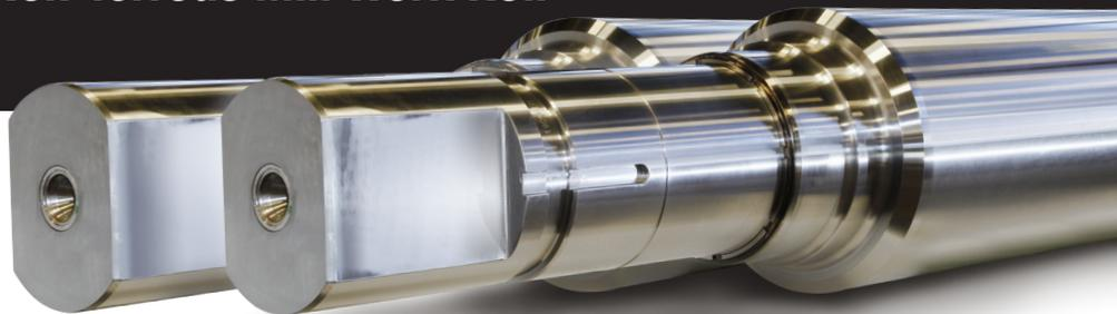
**U**nion Electric Åkers has revolutionized the hot rolling of nonferrous products by the development of our hot working die steel roll - 5CR80MO. Developed to provide a unique combination of superior high temperature thermal fatigue and wear properties, this alloy will provide an improvement to your overall roll performance and mill throughput. Our 5CR80MO roll has become the proven and established “roll of choice” for the majority of the world’s largest hot rolled non-ferrous producers.
